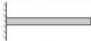
Figure 33: Uniform cylindrical rod fixed at left end.
